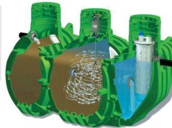
If regulations in your area are demanding nutrient reduction for onsite treatment and disposal systems and you have difficult access conditions, consider the Singulair Green Tank. Our Green tank option weighs 900 pounds and offers the same Total Nitrogen Treatment and volume as our standard concrete models. We also manufacture concrete dead men for anti-buoyancy purposes. You can rely on Norweco, the leader in advanced treatment unit technology.
