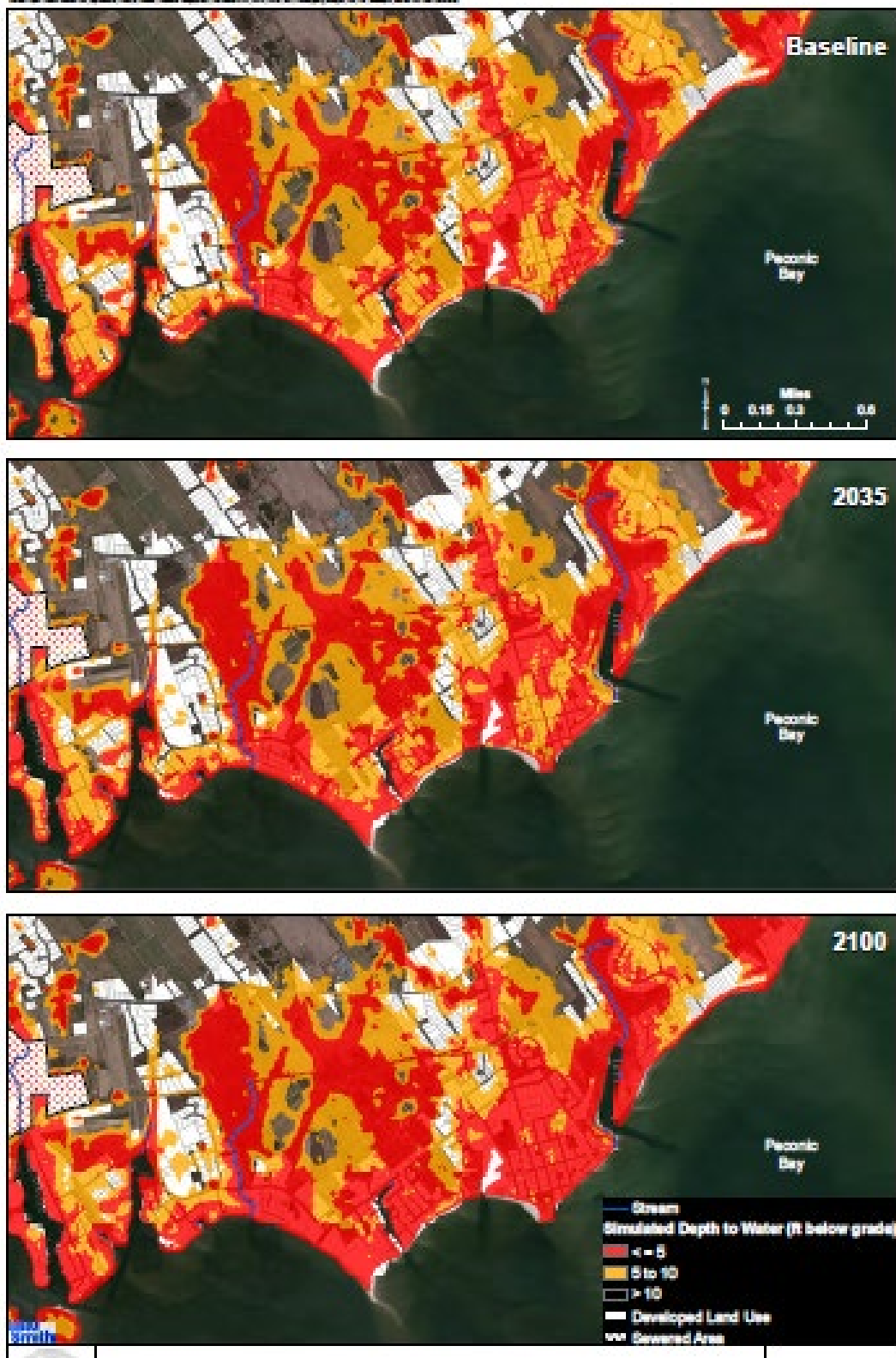
Figure 8-15 Simulated Impacts of Sea Level Rise on the North Fork Water Table (Source: 2015 Comp Plan)
